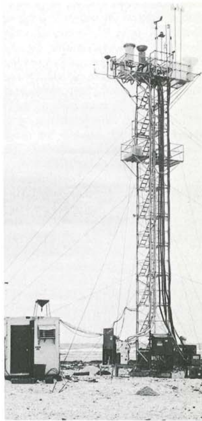
Long-range transport. On a remote atoll in the western Pacific, this tower collects wind-borne particles falling into the ocean from predetermined directions. Results from the tower recorded the subsidence of an Asian dust storm through the 100-fold decline from April to August 1979 in aluminum-containing dust. For comparison, the concentration of sodium, which is derived from sea spray that is always present, remains constant.
