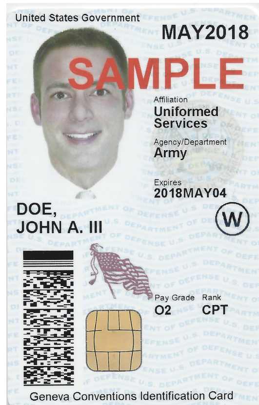
Figure 2- The Common Access Card (CAC) is the standard identification for the U.S. Department of Defense. The CAC is a “smart” card and is also used to access to buildings, controlled spaces, as well as the DoD computer network and systems. It stores information on four layers: 1) the card itself, with readable information and images printed on the card, the barcodes and magnetic strip, 2) the RFID antenna embedded in-between the layers of the card, 3) the antenna provides contactless physical access, such as buildings and doors, and 4) the chip, which is used for computer login, two factor user authentication, and document signing.
