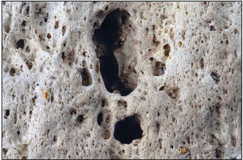
Figure 5.9: A close-up of a pumice stone, revealing its highly porous and vesicular texture. These gas bubbles make the rock so lightweight that it is able to float. Field of view is 2.7 centimeters (1 inch) across.
