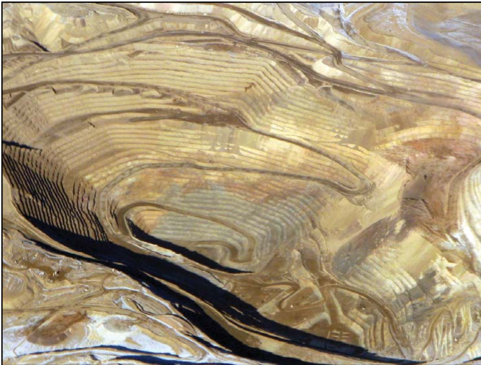
Figure 5.4: An aerial view of Round Mountain gold mine, an open pit mine in Nye County, Nevada. Round Mountain existed as an underground mine beginning in 1906, eventually being converted to an open pit sixty years later. The pit is about 2500 meters (9200 feet) wide and 1493 meters (4900 feet) deep.
