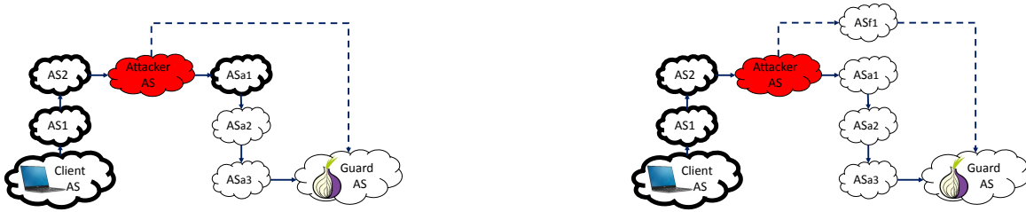
Fig. 4. Example scenarios of shortest path attack, where the attacker AS (highlighted in red) sends false announcement to its neighbors to attract traffic. The actual path from the attacker AS to the guard AS is denoted by solid lines, and the fake paths announced by the attacker are denoted by dashed lines. The ASes that are influenced by the false announcement are highlighted in bold.
