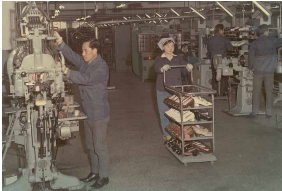
Heel lasting in the Kumkang Shoe Manufacturing Company, Ltd. Plant in Korea—a KDFC financed project
