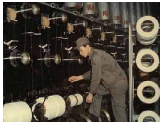
Take-up process in polyester staple fiber production of the Daehan Synthetic Fiber Company, Ltd
