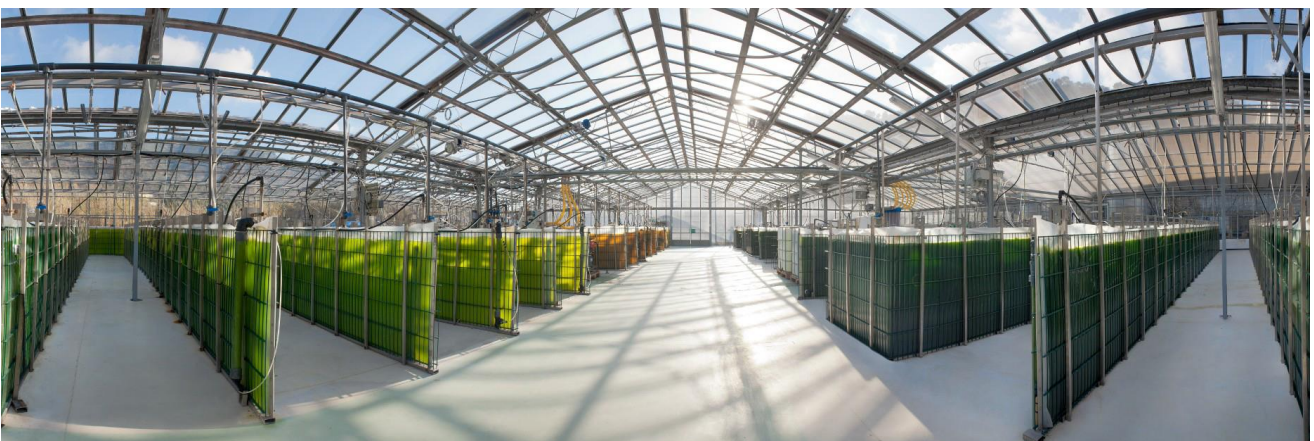
Figure 6: Photobioreactor microalgae production © Archimede Ricerche, 2018 For reproduction or use of this material, permission must be sought directly from the copyright holder.
