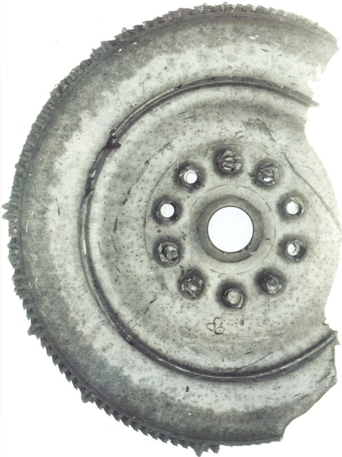
G-OJEM'S NO 2 ENGINE HP TURBINE DISC PORTION
