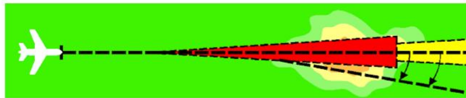
Figure 1: TAWS protective envelope formation for direct horizontal flight
