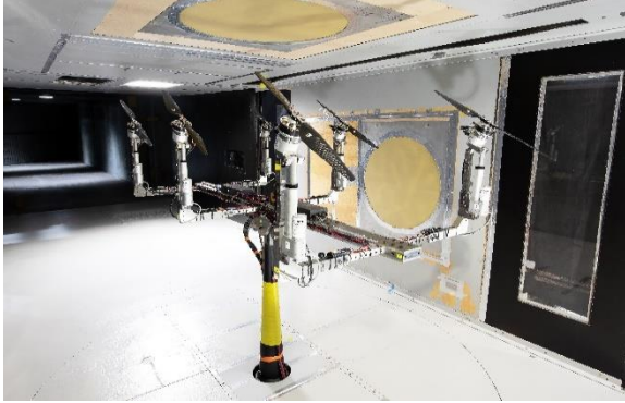
Figure 1.1 MTB in the U.S. Army's 7-by 10-Foot Wind Tunnel at NASA Ames Research Center.
