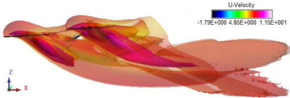
Figure 4.2 Flow visualization (showing U-velocity in m/s) of RotCFD simulation for original quad case, 20 ft/s tunnel speed, 0 deg pitch angle, with the quadrotor fuselage in the tunnel.
