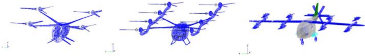
Figure 1. OpenVSP model showing rotor configuration: Quadrotor, Octocopter, and LPC.
