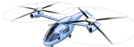
Figure 2. Six-passenger side-by-side helicopter with hybrid propulsion.
