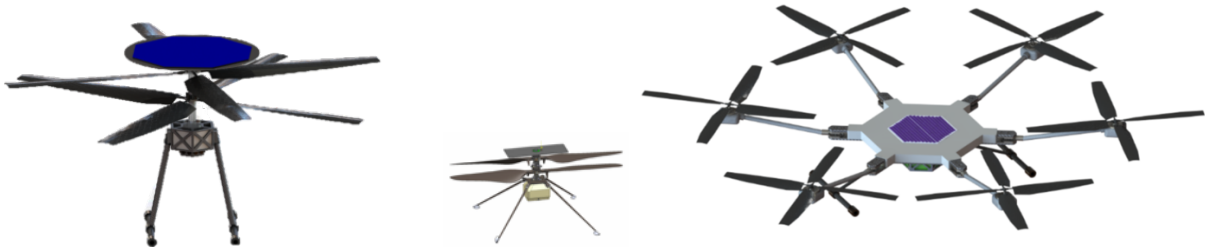
Figure 7. Mars Science Helicopter configurations, with Mars Helicopter (center) for scale.
