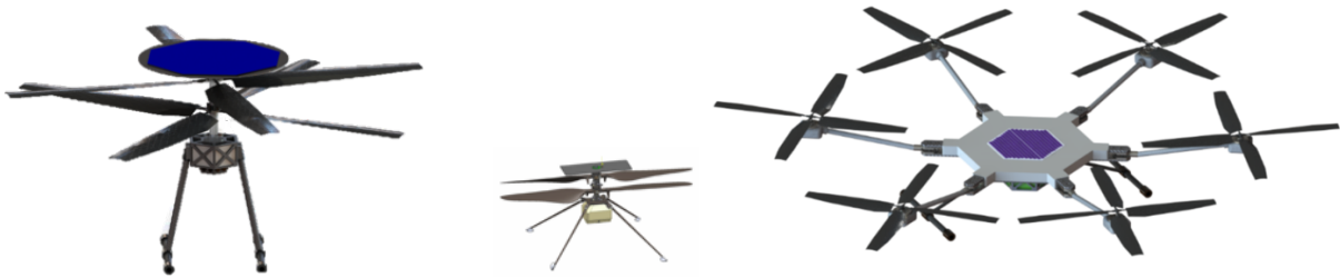
Figure 19. Mars Science Helicopter configurations, with Mars Helicopter (center) for scale.
