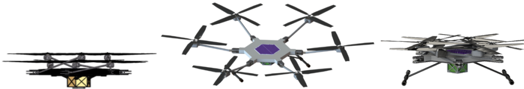
Figure 23. Mars Science Helicopter in hexacopter configuration, folded and unfolded.
