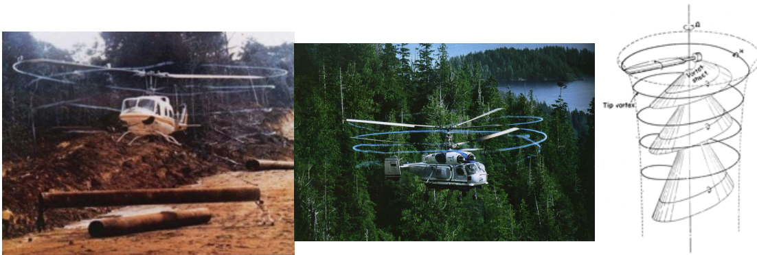
Figure 4. Rotor wake geometry structure in hover.
