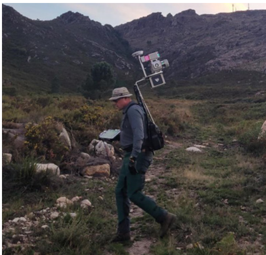
Mountain forest survey with a dual-wavelength backpack laser scanning for modeling and assessing forest fire risk in Xures national park, Galicia, Spain. (Image: Lino Orion)
