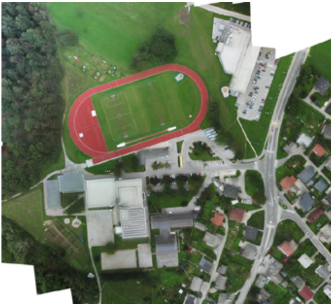
Figure 5: Orthophoto of the school area in Radovljica, created out of DŠGS FlyEye aerial images.
