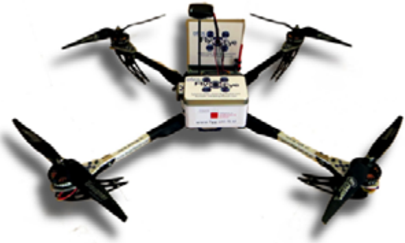
Figure 1: DŠGS FlyEye quadcopter equipped with digital camera mounted in aluminum case in the front.
