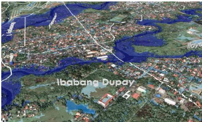
Figure 2. Snapshot of a flood simulation from animation, blue areas showing the possible extent of flood inundation (from https://dream.upd.edu.ph/products/flood-hazard-maps/ )
