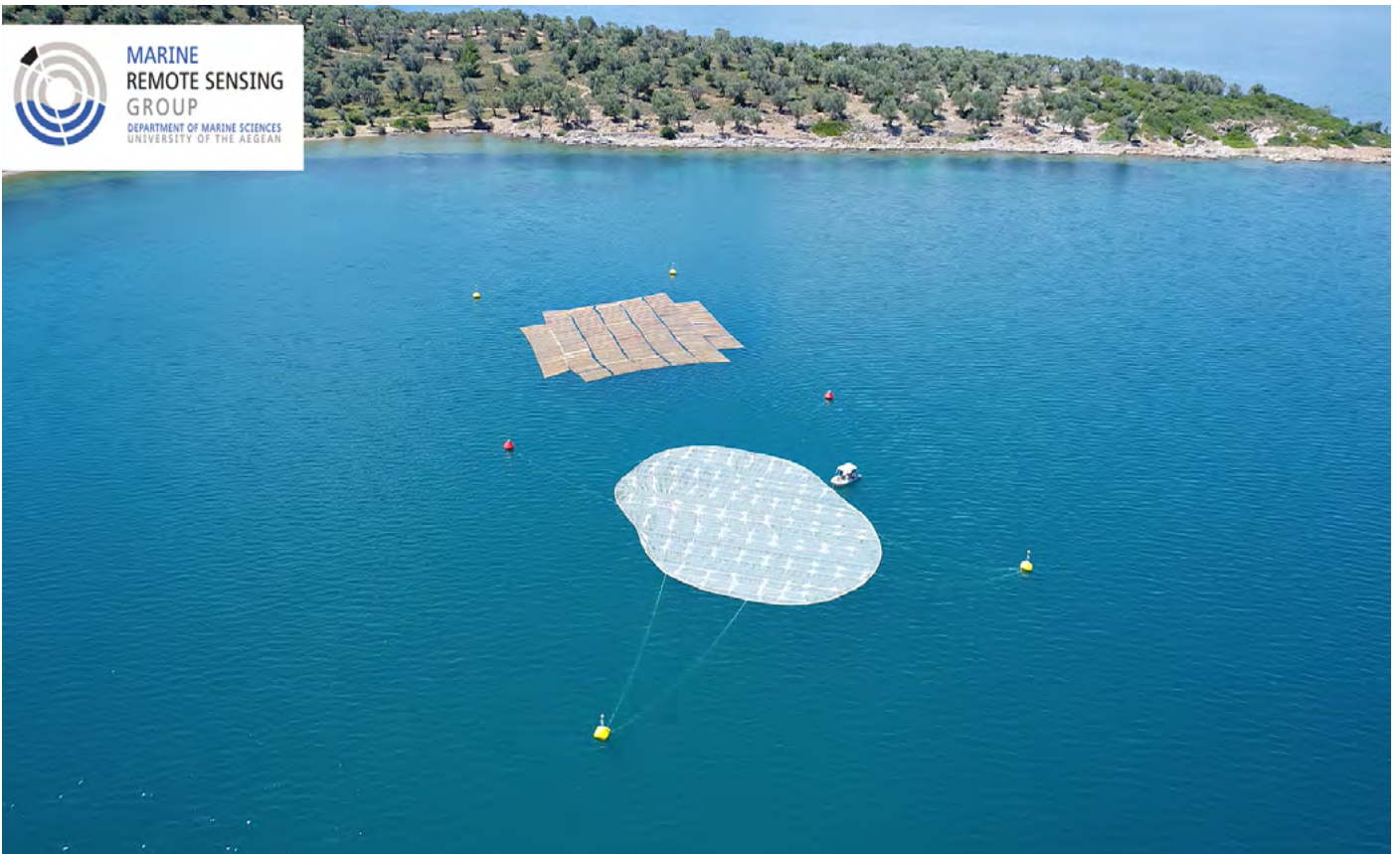
Figure 2. UAS image of deployment area showing HDPE mesh and wooden targets, dated: 21/06/2021.
