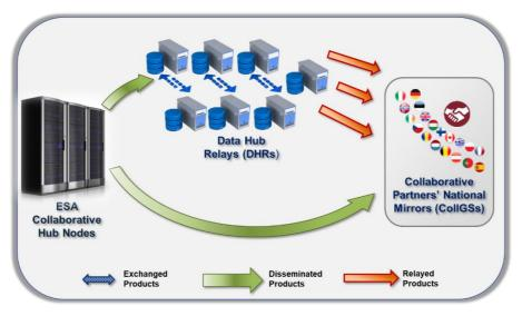
Figure 66: Schematic showing general data flow of user-level data from the Collaborative Data Hub to the Collaborative National Mirrors, highlighting the terminology used.
