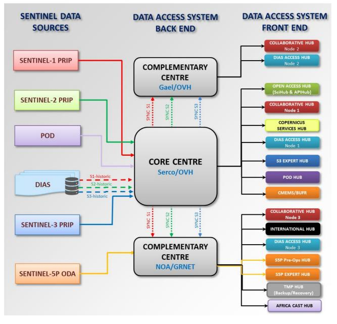
Figure 4: Data Access System Physical Architecture Overview during Y2023.
