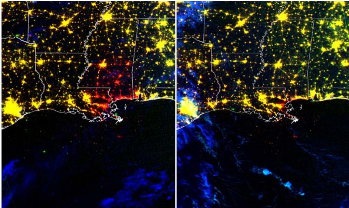
Figure 13. Affected area (show in red) of blacked out lights during hurricane Katrina with the 2004 Annual Composite vs. August 30, 2005 local time on the left and the 2004 Annual Composite vs. Sept. 11th local time on the right.
