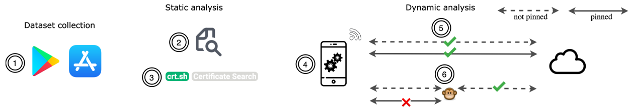
Figure 5.1: Our methodology to detect certificate pinning. We (1) crawl Android and iOS apps, (2) search app contents for certificate files or hashes, (3) retrieve certificates corresponding to the hashes using publicly available Certificate Transparency logs, (4) launch every app on a real device and collect network traffic in two distinct settings: (5) when app traffic is not intercepted, and (6) when app traffic is intercepted through monkey-in-the-middle (MITM) technique. We identify and mark TLS connections that transmit data in the former setting but not the latter as pinned.
