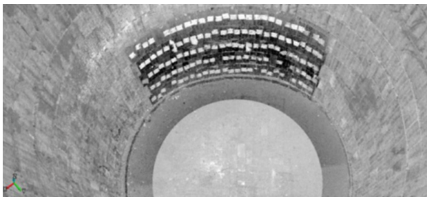
Figure 5. HML assembled with AS-K brick in the wall in a 3D view.
