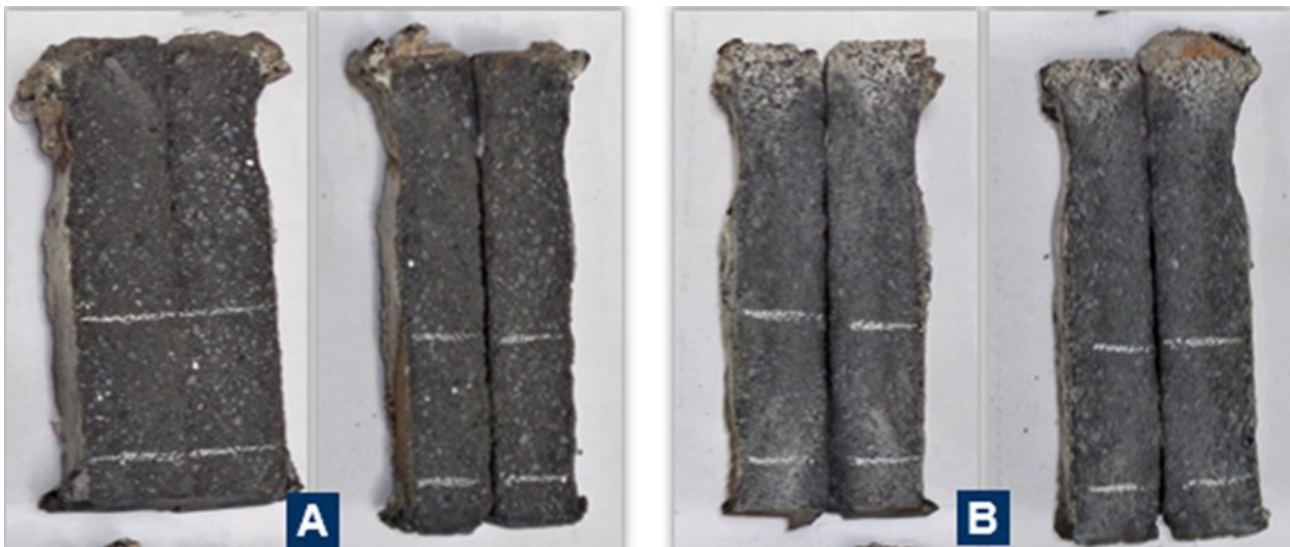
Figure 3. Images after corrosion test: A) ASC brick and B) AS-K brick.
