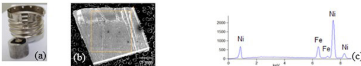
Figure 1. (a) Photograph of a socket of one type of bulb LED lamp, (b) micrograph of one piece of the socket, obtained by SEM, and (c) EDS spectrum of the region indicated in orange in figure b.
