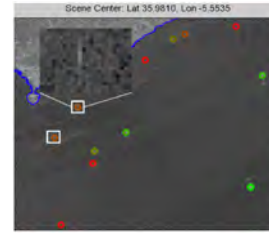
Fig. 3. SIDECAR: snapshot of the ship detection report and coastline isolation (blue line). Confidence is colour-coded from red (0 – minimum) to green (1 – maximum).
