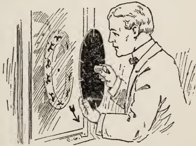
Holding a phenakistoscope before a mirror and ready to twirl it around.
