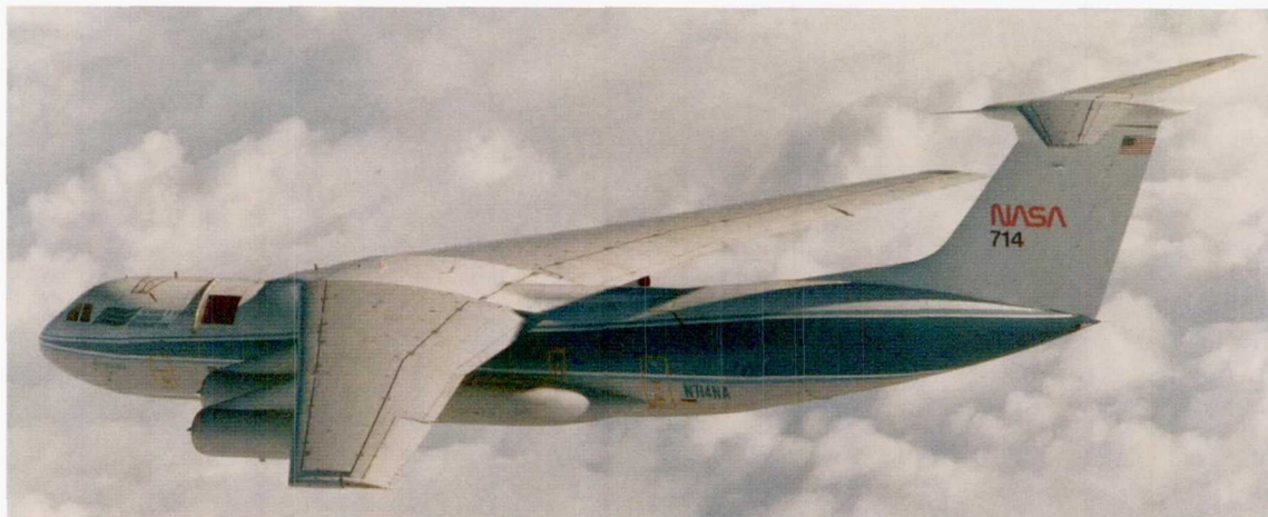
The Kuiper Airborne Observatory (KAO), a unique infrared astronomical facility operated by NASA. Flying at altitudes above most of the terrestrial atmosphere, the KAO permits studies to be made in parts of the spectrum that are inaccessible to ground-based telescopes. Observations from the KAO's 1-meter telescope were important in establishing that Saturn has an internal heat source and in probing the upper atmosphere of Titan.
