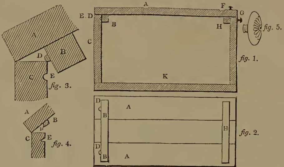
*Fig. 1.* Section of the box. *A*, the lid. *K*, the bottom. *C*, the side.
