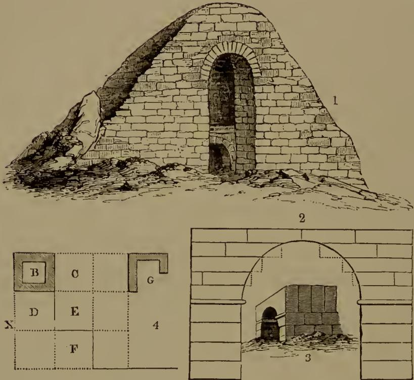
No. 427. *Fig. 1.* Vaulted rooms and doorway of a crude brick pyramid at Thebes.
