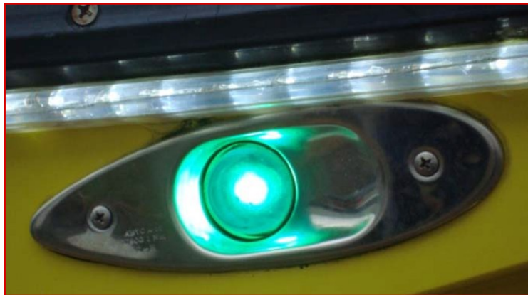
LEDs under rub rail surrounding vessel.
