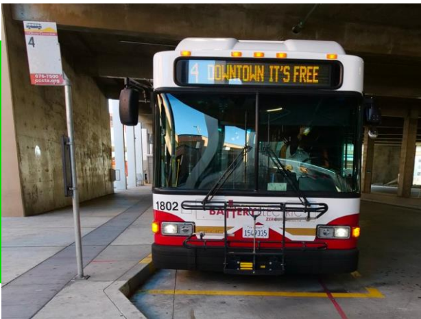
CCCTA Gillig Battery Electric Bus charging on WAVE charging pad.
