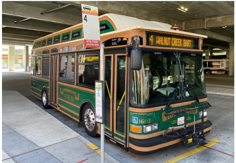
Gillig Trolley Replica Electric Bus on WAVE charging pad - Walnut Creek BART Station.
