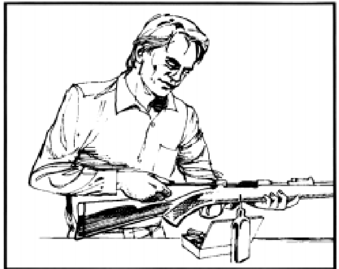
Cleaning a firearm, the rod being inserted from the chamber end of the barrel.
