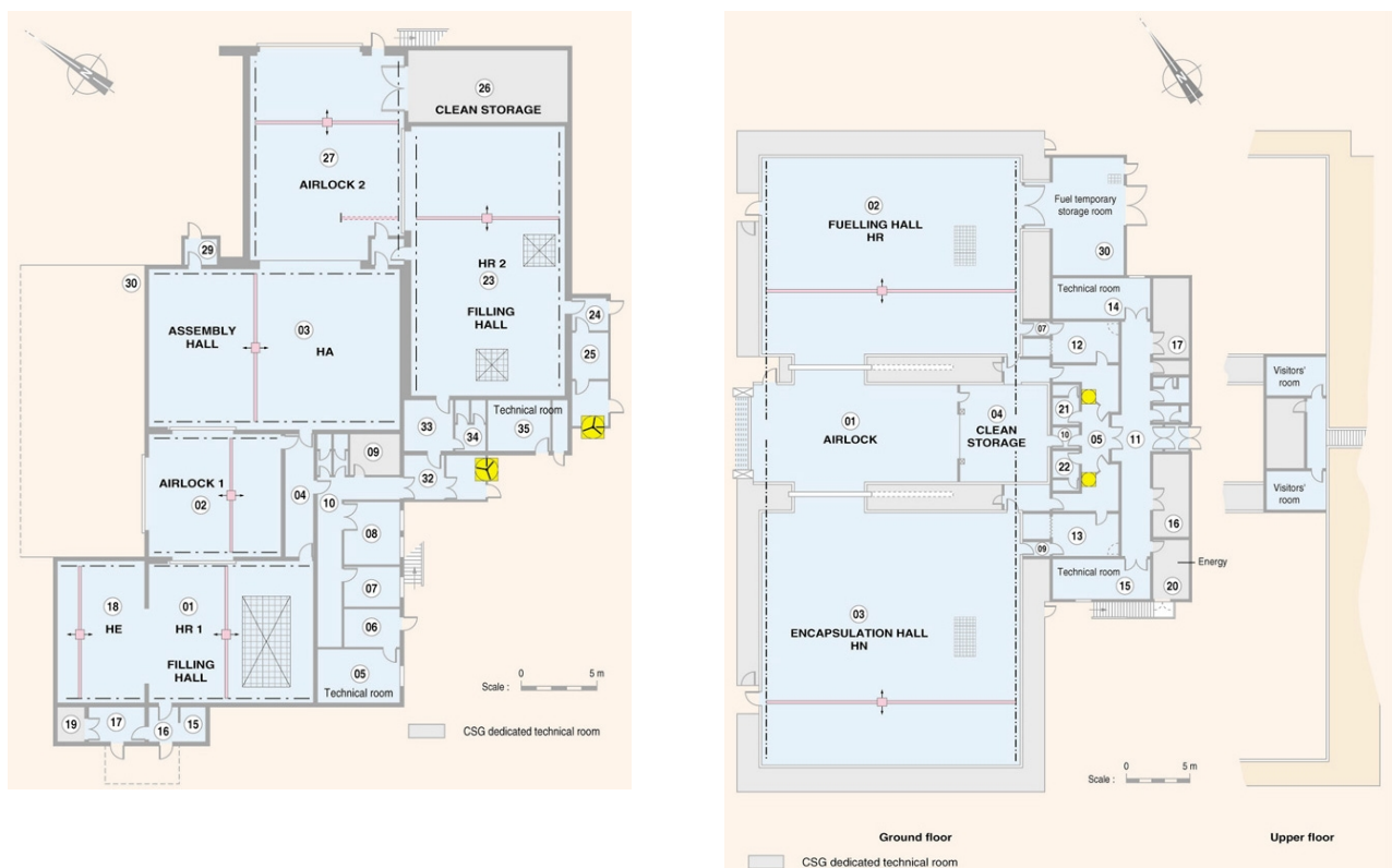
Figure 6.9 – Layout of Hazardous and Upper Composite Integration Facilities at S3 area (S3A and S3B)
