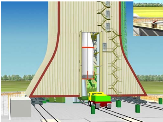
Payload composite hoisting on Launch Vehicle
