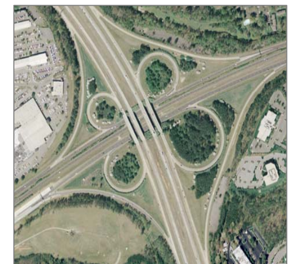
Cloverleaf interchange configuration
