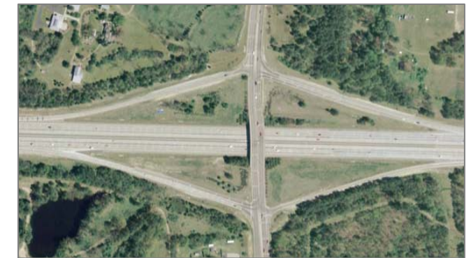
Diamond interchange configuration
