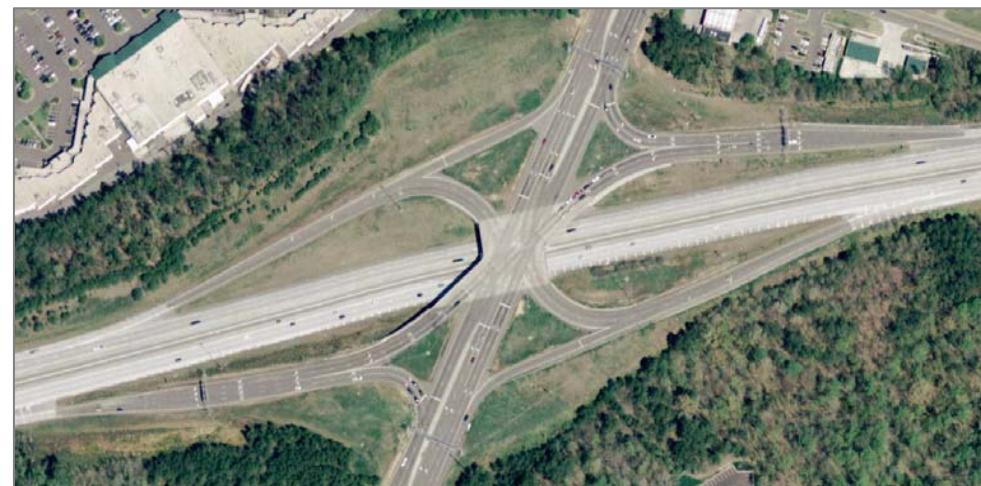
Single point urban interchange configuration
