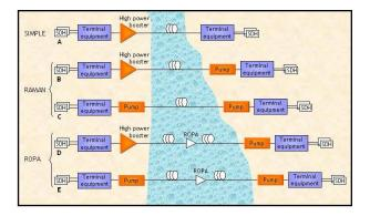
Figure 1: Optical amplification configurations
