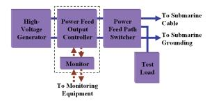
Figure 3 Block Diagram of NPF Series PFE
