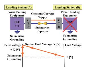
Figure 2 Power Feeding Balancing in Case of a PFE Failure
