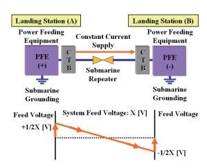
Figure 1 Power Feeding Configuration with Dual-End Feeding
