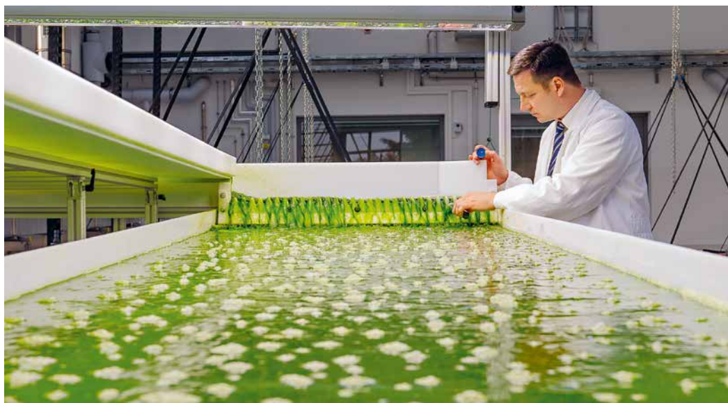
Professor Thomas Brück at an open photo-bioreactor. The promising organisms are cultivated in these types of basins
