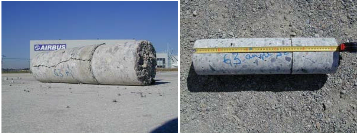
Figure IV-37 : Slab 63 – Core sampling.
