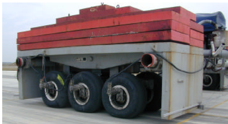
Figure III-8 : Details of the B777 six wheels bogie.
