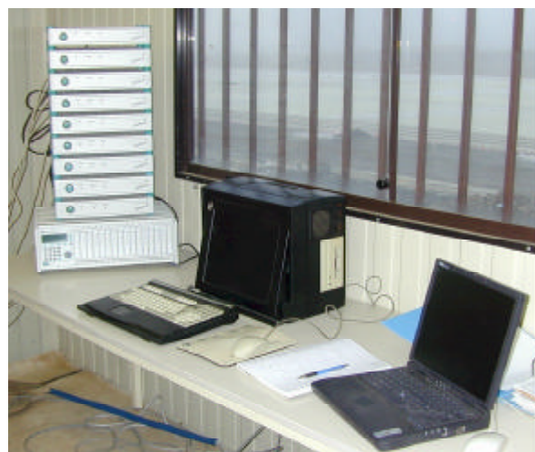
Figure II-22 : Acquisition unit, MGCPlus & Spiders.
