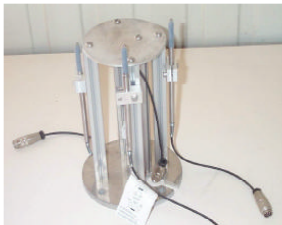
Figure II-3 : Solartron LVDT sensors on their frame.
