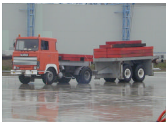
Figure III-3 : B747-400 bogie hauled by the Service truck of STBA.
