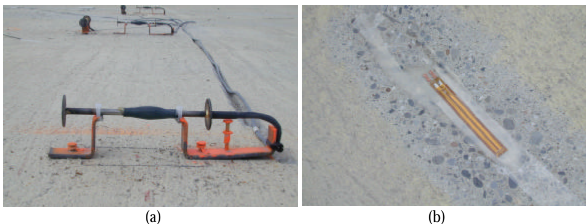
Figure II-1 : (a) sensor and support / (b) strain gauge.
