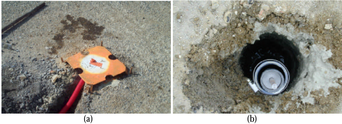
Figure II-4 : (a) Frame attachment plate / (b) Reference rod.
