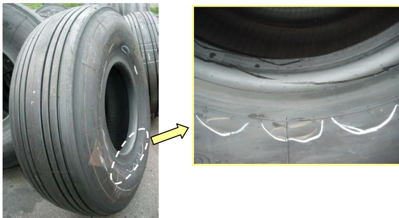
Figure 3: Bulges at bead area
