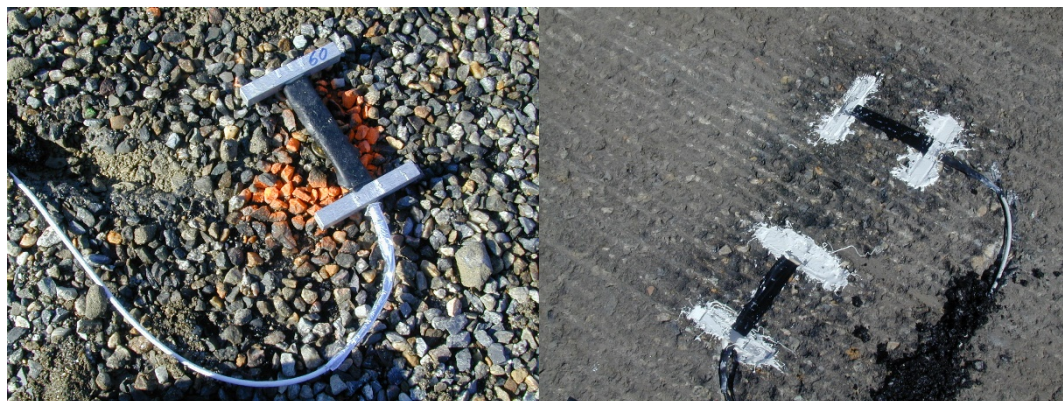
Figure 31: Horizontal strain gauges
