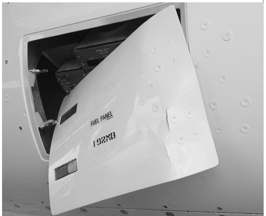
Damage to a fuel panel following incomplete latch engagement
