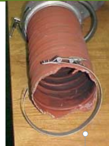
Example of a failed clamp
