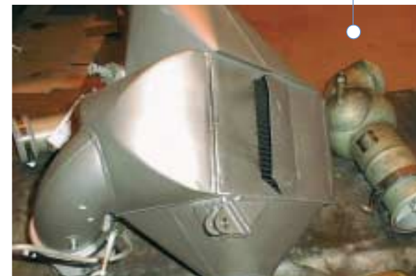
Example of a ruptured condenser
