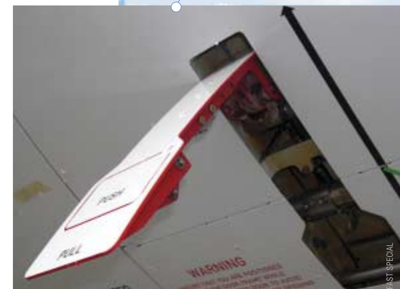
New standard door handle from production aircraft
