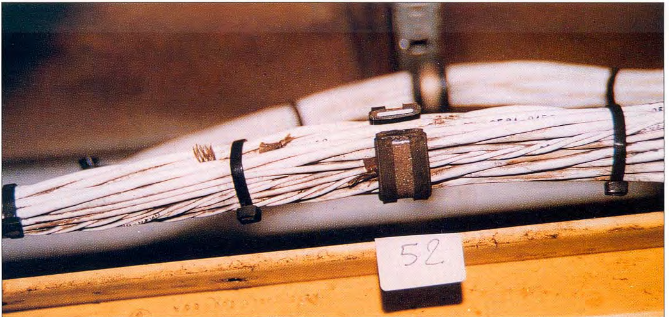
This clamp has sheered right off and the harness is now unsupported.
