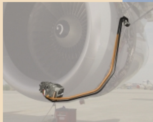
The oil circulates outside the IDG, into the cooler...
