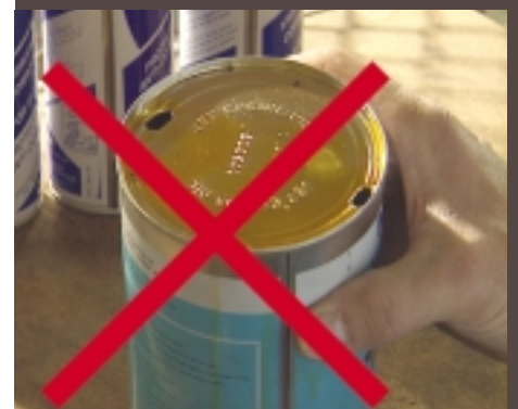
Never use a can that has been already opened when servicing the IDG!
