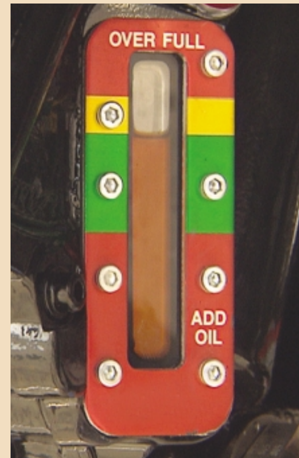
The optimum oil level is at or near the top of the green band.
