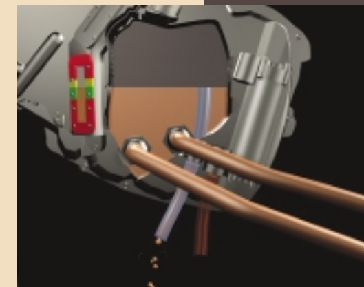
The top of the overflow stand pipe corresponds to the top of the green band of the sight glass
