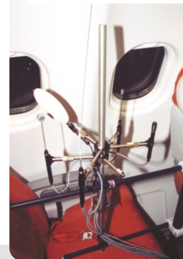
Air conditioning measurement device
