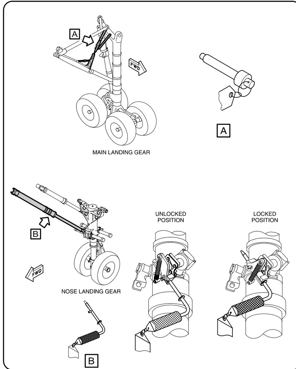
Landing Gear Ground Lock Safety Pin - Installation
