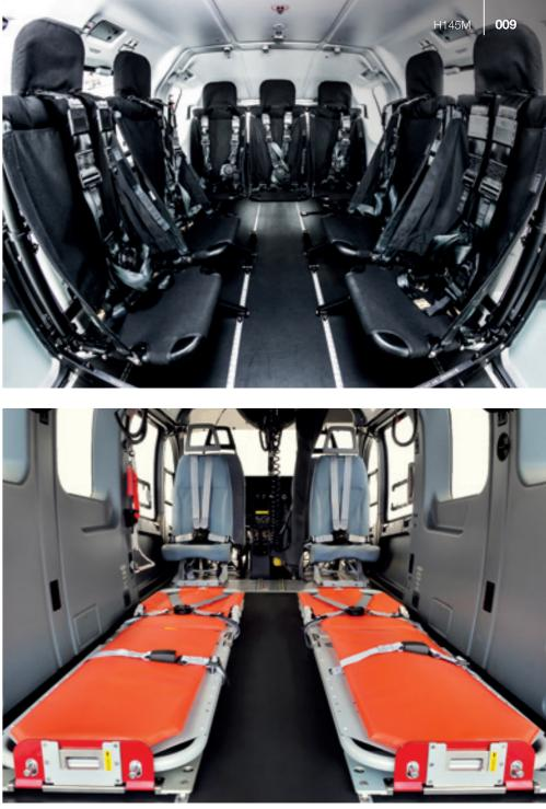
No matter what the emergency, the H145M quick role change concept allows to easily and quickly fit its flat floor with a wide range of available equipment.
