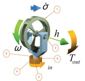
The kinetic momentum is fulfilled by the wheel (1) at constant speed. The precession of the wheel is fulfilled by the gimbal motor (2). The output loads are supported by the ball bearing of the wheel (3) and of the gimbal (4). An angular encoder allows the measurement of the gimbal position (5). The signals and power are led to the wheel through sliprings (6).
