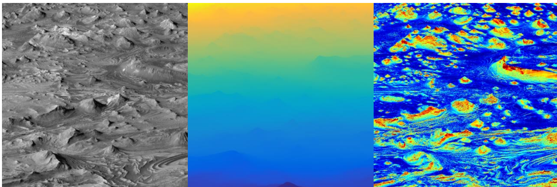
Fig. 8: Synthetic image of the surface of Mars generated with SurRender (left) using MRO/HiRISE images and DEM and the associated depth map (center) and slope map (right).
