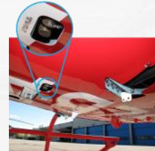
H130 ELECTRICAL CONTROLLER FOR 50AMP/ LONGLINE/CAROUSEL
