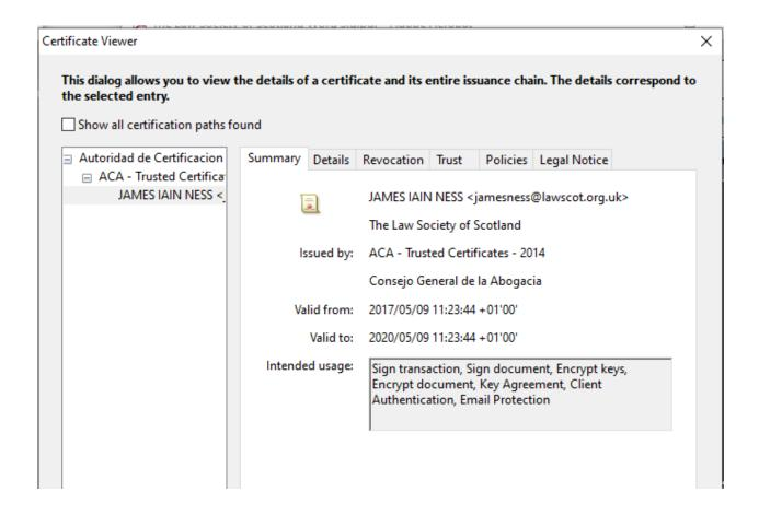
You can also see what's called an "issuance chain" on the left hand side. The signature you are looking at is based on an underlying certificate issued by ACA. That in itself is based on a root certificate - the top entry. This is the one that needs to be trusted in your Adobe version on your computer. Once done, every other signature based on the same root, i.e. every other Smartcard signature, will also be trusted in your system.
