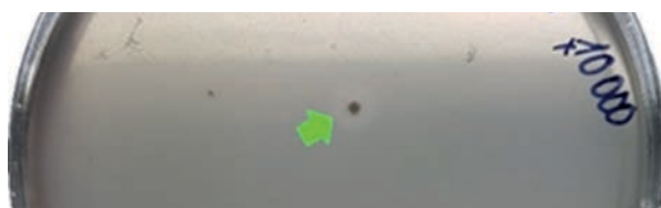
Fig. 2. Hydrolysis zone formed by Rhodococcus sp. on a selective growth media containing polyether polyurethane. Bacteria was isolated from Lithuanian soil.
