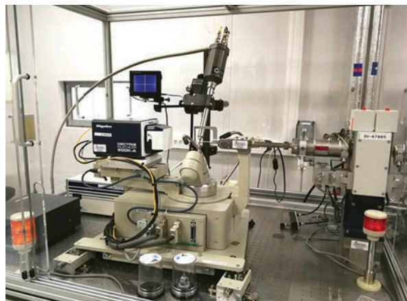
Fig. 1 b. An X-ray diffractometer for small molecule and macromolecule crystal determination.
