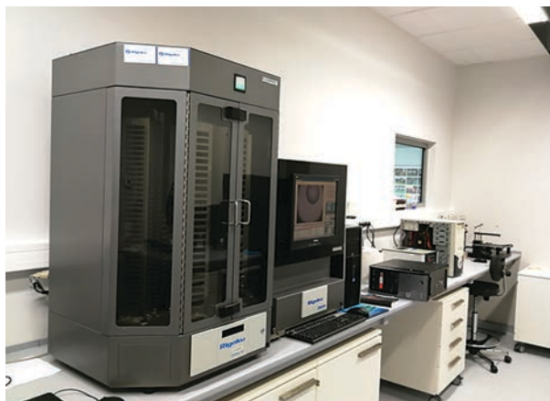
Fig. 1 a. Robotic equipment for crystal growth and automatic crystal observations; a crystallization plate preparation robot (in the back).
