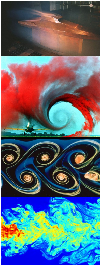
q / Fluid friction depends on the fluid's pattern of flow, so it is more complicated than friction between solids, and there are no simple, universally applicable formulas to calculate it. From top to bottom: supersonic wind tunnel, vortex created by a crop duster, series of vortices created by a single object, turbulence.
