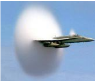
ab / As in figure aa, this plane shows a shock wave. The sudden decompression of the air causes water droplets to condense, forming a cloud.
