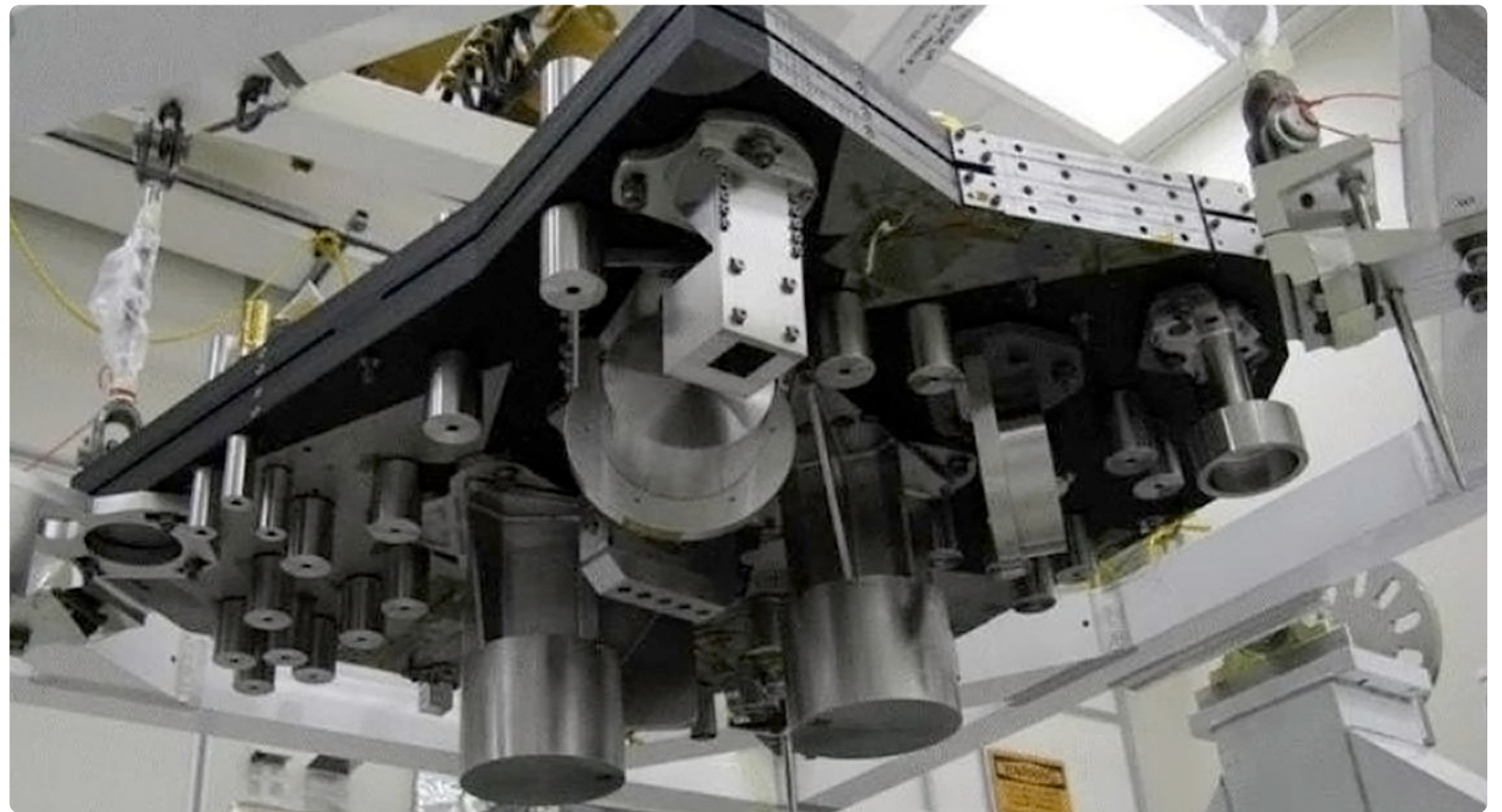
A test piece of the Near-Infrared Camera optical bench is prepared for stress testing.
